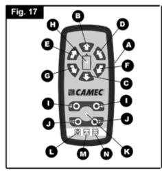
After successful synchronisation, the green LED on the control unit (Fig. 16B) and on the remote control handset (Fig. 17H) will illuminate continuously.
